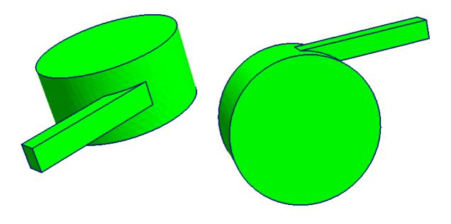
2) Tangential Inlet Angled to Cylinder Lid – problems fabricating in  ${\tt gmsh}$
